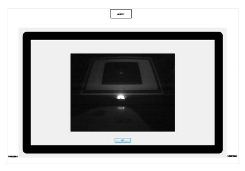
**7.5.3 Laser curtain alignment process** First rotate slowly #1 knob then you can see the reflection line like below picture
