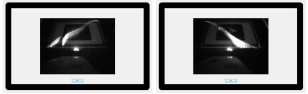
Then, rotating #2/#3 knob accordingly to make reflection line horizontal and near the laser module.
